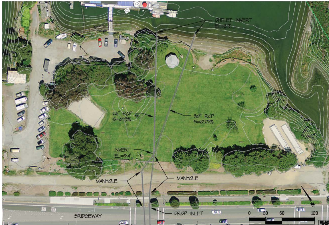
Figure 2. Dunphy Park Storm Drain Network
